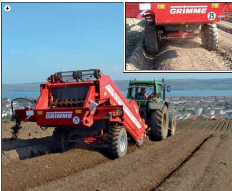
Well levelled: The hydraulic levelling adjustment (4) at the side keeps the machine horizontal on hillside located fields or in different furrow heights – for a constant even sieving and even ridge height. Additional option: the automatic levelling
