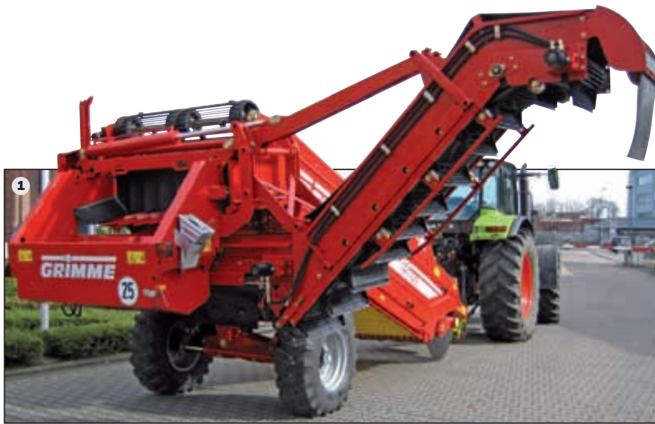
Unloading elevator: If stones and clods are unwanted in the furrow an unloading elevator (2 meter loading height) elevates to the right hand side (1).
