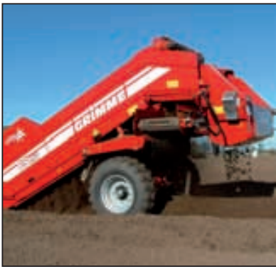
All models have a cross conveyor with 22 mm pitch as standard.
