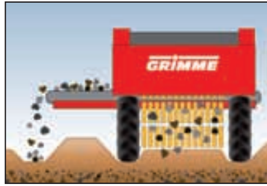
Phase 2: Bed separation with stone and clod separator of the CS/CW-series. The separator lifts the whole bed width and completely sieves the soil.
