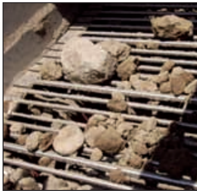
Every sixth web has a diameter of 16 mm. That gives you 3 important advantages: optimized soil transport on the webs, supported clod breaking and a higher stability of the web especially while transporting bigger stones
