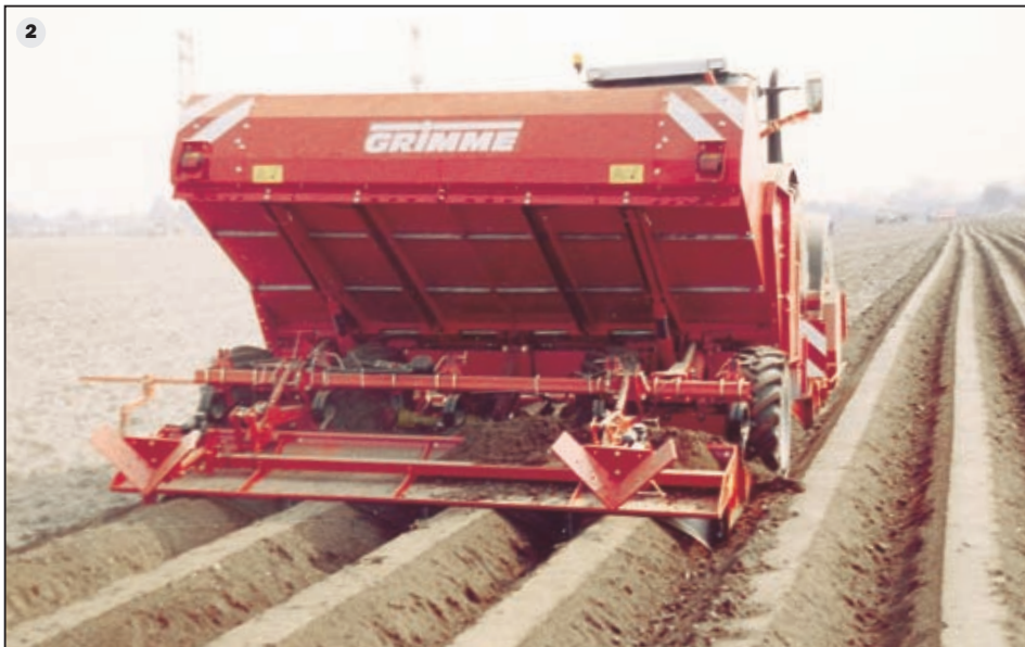
Optional extras that pay for themselves: with additional spring loaded ridging bodies and shaping board for planting and ridge shaping in one operation (2)
