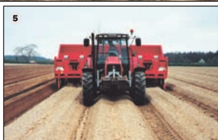
The alternative to the 2- and 4-row bed planting system: the high output 3-bed system, with a centrally pulled planter (5)
