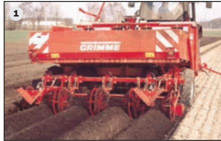
Solution for light soil: planter with additional spring loaded ridging bodies to shape ridges – including individually mounted, adjustable cage roller for light soils and better moisture retention (1)
