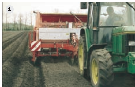
Solution: mechanical or hydraulically moveable drawbar (1)
