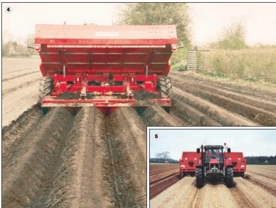
Big advantage: Because of the two large wheels (4) there are no wheelings in the beds. The following shaping hoods form the ridges.
