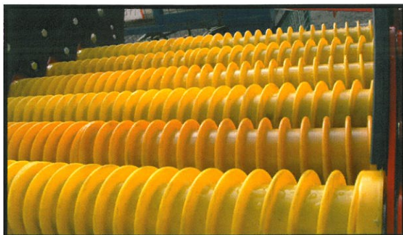
Polyurethane coils for gentle handling with effective cleaning
